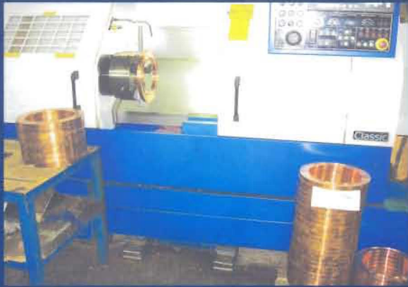
CNC Machining of Seam Welding Wheels
